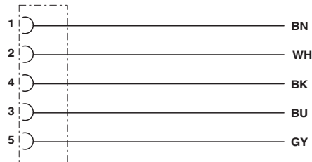
Contact assignment of the M12 socket
